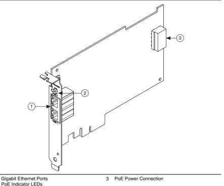
Figure 1. NI 8236 Connections and Indicators
